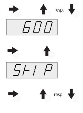
Press the key (5) and enter the temperature of 600°C using the keys (7) or (8). When the kiln reaches this temperature the TC60 will switch to the next ramp (section c).
