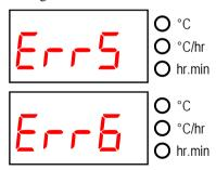
Error 5. Kiln temperature overshoot. The kiln temperature exceeds the desired temperature by at least 10°C / 20°C (installer selectable).
