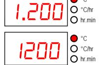
If the left-hand decimal point in the display is lit then the ST316 is locked. Press and hold in both the ♠ & ♣ keys for 5 seconds to unlock the ST316.
